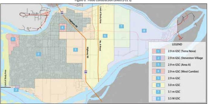
Figure 6: Flood Construction Levels (FCL's)
