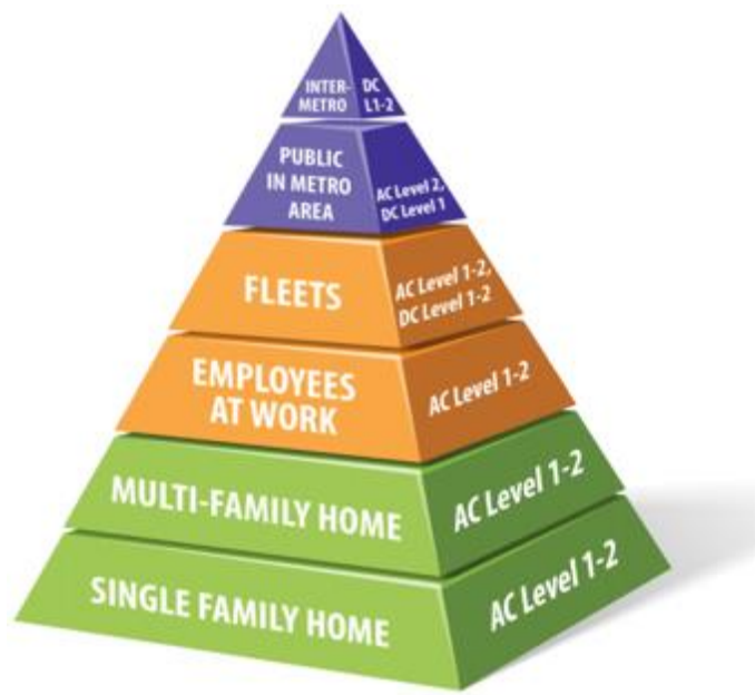
Figure 6: The charging pyramid 15 by Argonne National Laboratory demonstrates the hierarchy of electric vehicle charging location type frequencies. Electric vehicles are most frequently charged at home, where the vehicles are most often parked. Public charging, which has a comparatively lower demand, still plays an important role in the electric vehicle charging ecosystem.
