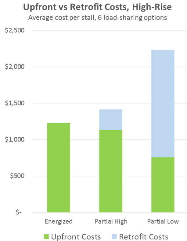
Figure 11: High-rise: electric vehicle supply equipment-ready (energized) infrastructure costs compared to two partial infrastructure options, split by upfront and future retrofit costs.
