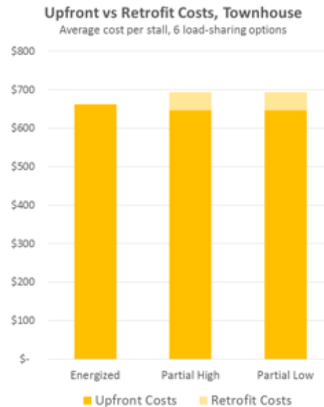
Figure 13: Townhouse: electric vehicle supply equipment-ready (energized) infrastructure costs compared to two partial infrastructure options, split by upfront and future retrofit costs.
