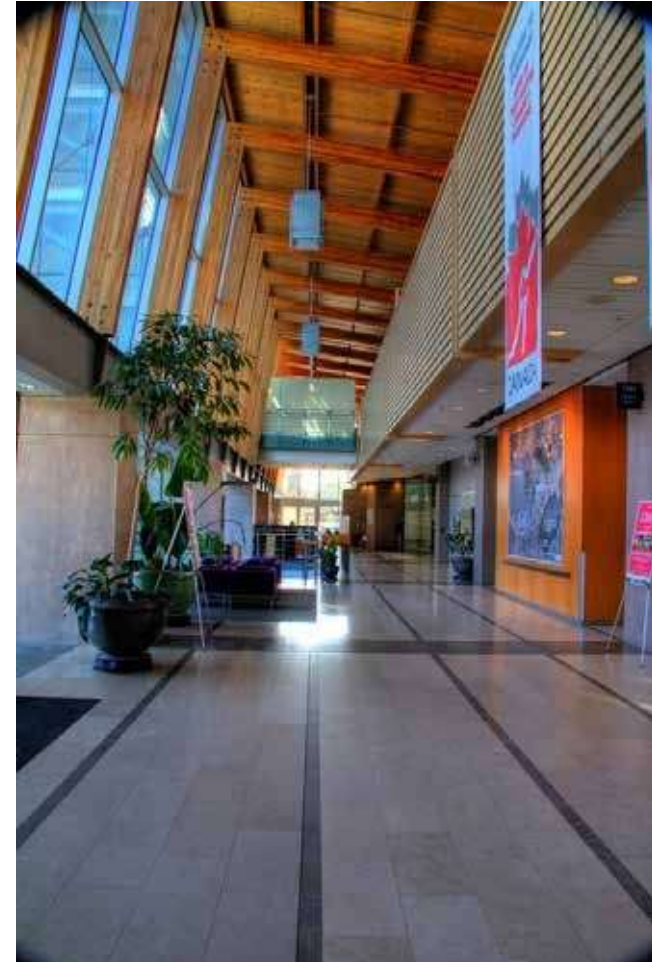
The disorienting effects of glare in public lobbies and hallways, can be reduced by using appropriate interior finish materials, and limiting adjacent large areas of glazing to north-facing exterior walls, as shown in this photo.
