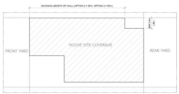
\* A continuous wall is defined as a wall without a minimum inward articulation of 2.4 m (8.0 ft.) or more from the minimum required side yard setback. The articulation must be maintained for a minimum horizontal distance of 2.4m (8.0 ft.) unless wall is discontinued.
