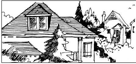
Create varied sloped – roof forms with frequent additive elements such as gables and dormers
